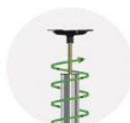
Seat rotation with RH height adjustment
